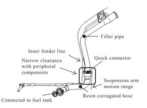
Fig. 6. Piping example using conventional resin filler hose
