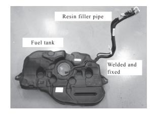
Fig. 3. Application example of resin blow-molded filler pipe
