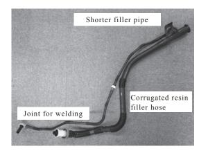
Fig. 4. Integral type resin filler neck hose
