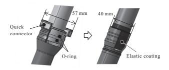
Fig. 7. Joining structure comparison with filler pipe
