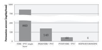
Fig. 5. Comparison between hose material configuration and fuel permeation amount
