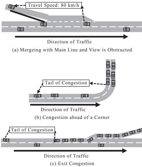
Fig. 1. Examples of use of information on travel speed and congested sections
