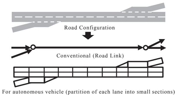
Fig. 2. Unit for generating and providing travel speed information
