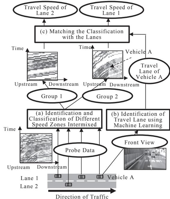
Fig. 3. System for generating lane-specific travel speed information
