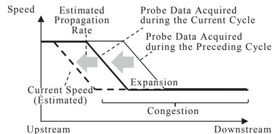
Fig. 4. Generation of travel speed information by estimating the propagation of traffic congestion
