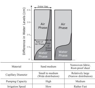
Fig.4. Ratios of the Air and Water Phases in the Irrigation Material for NSP
