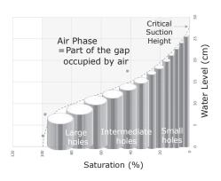
Fig.5. Capillary Diameter Distribution and Ratios of the Air and Water Phases
