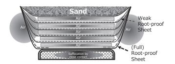
Fig. 10. Root Distribution of a Laminated Medium (Indicated with broken line)
