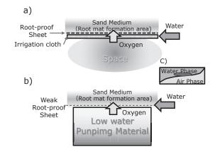
Fig. 11. Example of an Ideal Floor Irrigation Cultivation Method (schematic)a) Bottom of NSP; b) Layers of the laminated structure;c) Common environmental states
