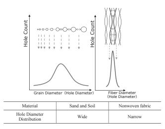
Fig.3. Irrigation Materials and Tube Diameter Distributions
