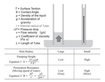
Fig.2. Relationship between Capillary Action and Irrigation Characteristics
