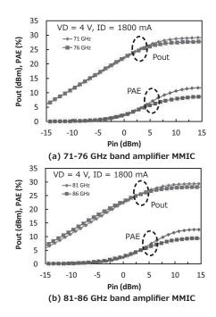
Fig. 8. Input-output power characteristics and PAE characteristics of the amplifier MMIC
