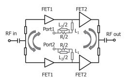
Fig. 3. Model simulating the stability of the unit amplifier
