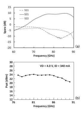
Fig. 5. Small signal characteristics (a) and saturated output characteristics (b) of the unit amplifier
