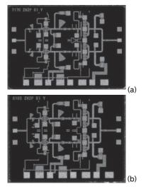
Fig. 1. (a) 71-76 GHz unit amplifier and (b) 81-86 GHz unit amplifier
