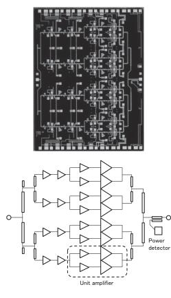
Fig. 6. Photo and block diagram of the amplifier MMIC
