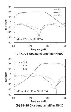
Fig. 7. Small signal characteristics of the amplifier MMIC
