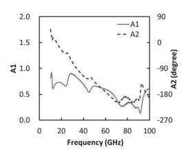
Fig. 4. Simulation results of the stability of the unit amplifier
