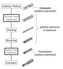
Fig. 3. Manufacturing processes for aluminum wire
