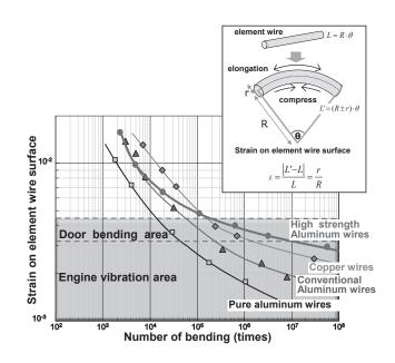
Fig. 5. S-N characteristics of various conductors
