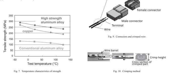
insulating oxide film, it needs to be swaged stronger than copper to obtain stable contact resistance. We investigated the physical properties of the high-strength aluminum wire conductor in terms of connection performance and verified whether the crimping method used for conventional aluminum wire can also be used for the developed wire. The results are shown in Table 3.
