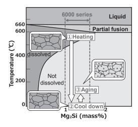
Fig. 4. Pseudo-binary phase diagram for Al-Mg<sub>2</sub>Si
