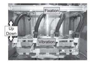
Photo 2. Situation of tests simulating engine vibration
