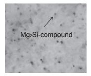
Photo 1. Finely dispersed Mg2Si intermetallic compounds
