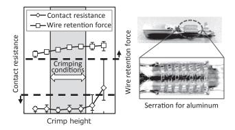
Fig. 11. Crimping characteristics of terminals for high-strength aluminum wires
