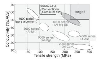
Fig. 1. Characteristics of various aluminum alloys
