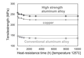
Fig. 8. Strength after high temperature storage
