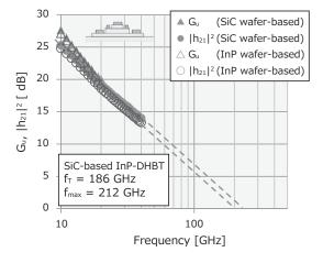
Fig. 7. High-frequency characteristics (single-emitter)
