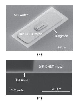
Fig. 2. SEM images (a) InP-DHBT mesa formed on SiC wafer (b) Cross section of bonding interface
