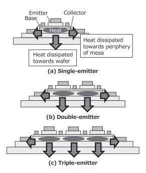
Fig. 4. Rendered image of heat dissipation paths
