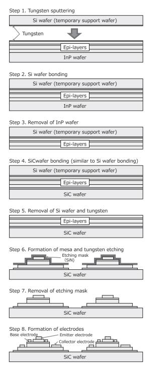
Fig. 1. Fabrication process
