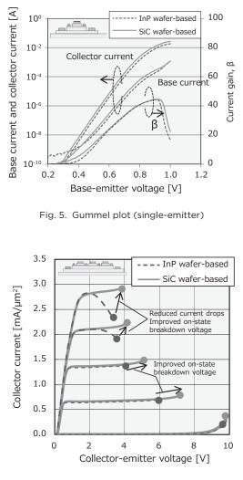
Fig. 6. Common emitter current-voltage characteristics (triple-emitter)
