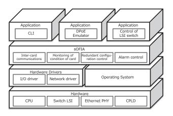
Fig. 2. Hierarchical structure of access equipment software
