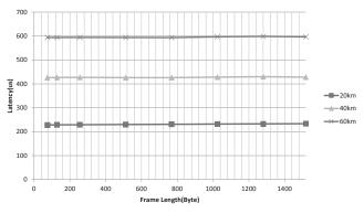
Fig. 4. Latency with a 10G repeater
