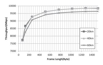
Fig. 3. L2 throughput with a connected 10G repeater
