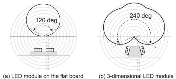
**Fig. 6.** Calculation result of the light distribution
