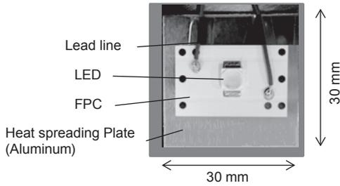
Photo 1. Test LED module for evaluating the cooling performance
