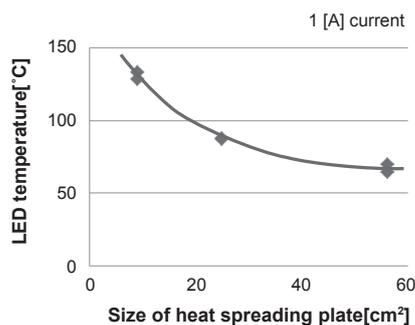
**Fig. 7.** Evaluation result of the cooling performance for the high output LED
