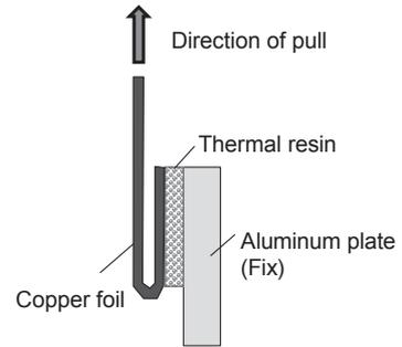
Fig. 3. Test piece and measuring method
