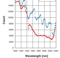
(c) Reflectance spectra of hydroxypropyl cellulose (HPC) and ascorbic acid
