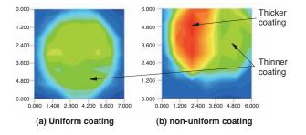
Fig. 5. Image of thickness of magnesium stearate coating (This figure is result of collaborative work with prof. Ozaki group in Kwansei Gakuin Univ.)
