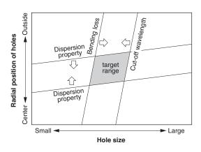
Fig. 1. Relationship between hole structure and optical properties
