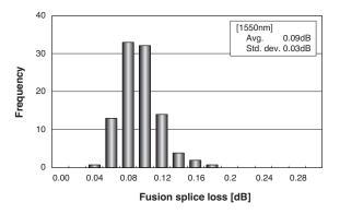
Fig. 5. Histogram of fusion splice loss between SM-HAFs
