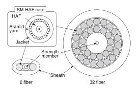
Fig. 7. Cross section of SM-HAF cable
