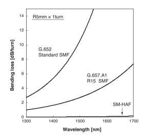
Fig. 2. Comparison of wavelength dependence of bending loss
