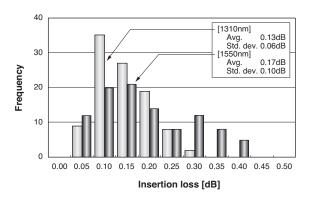
Fig. 6. Histogram of SM-HAF patch cord insertion loss
