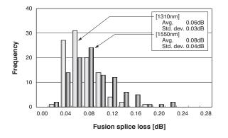
Fig. 4. Histogram of fusion splice loss between SM-HAF and SMF
