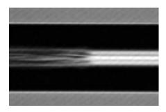
Photo 2. Side view around fusion splice point
