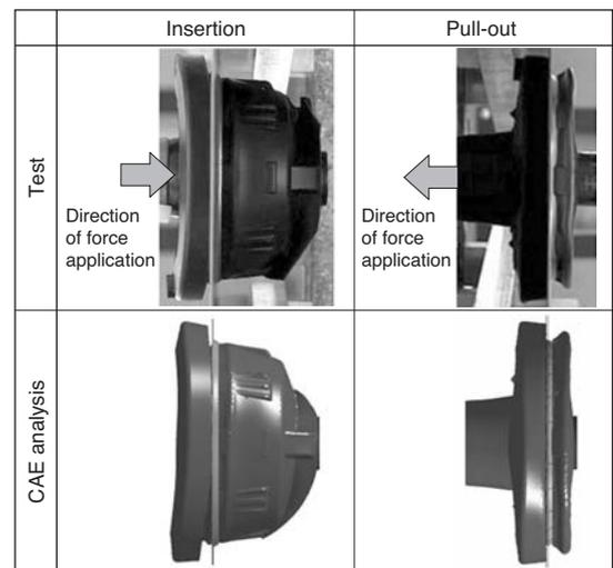
Fig. 10. Deformation comparison (under peak loads)
