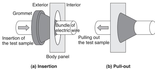
Fig. 1. Schematic illustration of test
