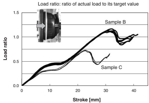
Fig. 9. Insertion force comparison
