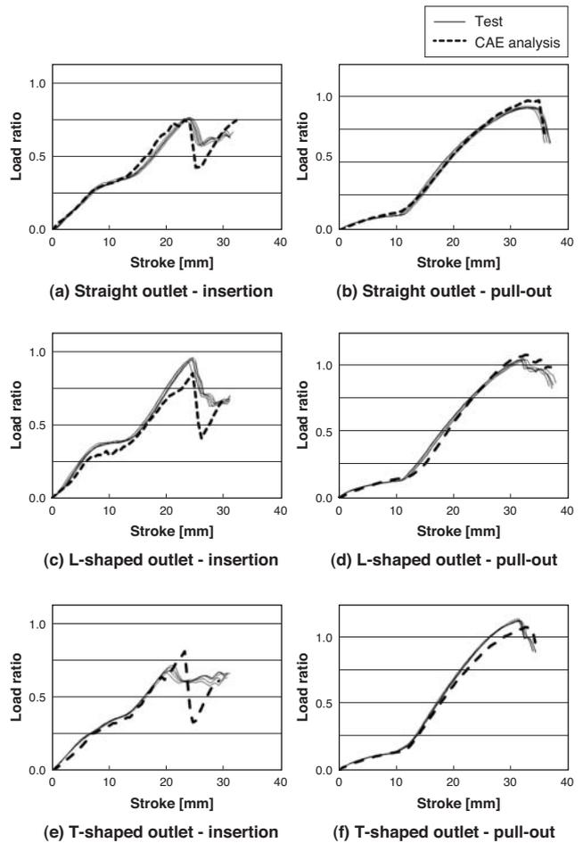
Fig. 13. Load ratio/stroke curve comparison
