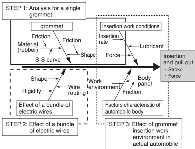
Fig. 4. Cause-Effect Diagram (insertion and pull-out)
