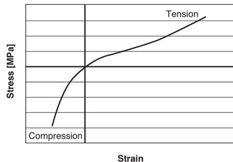
Fig. 6. S-S curve of rubber material
