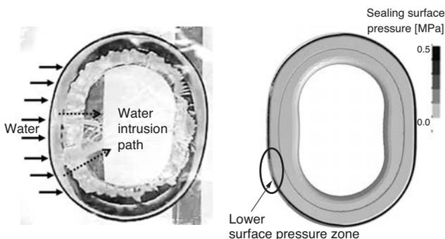
**Fig. 15.** Water intrusion path (water injection)
