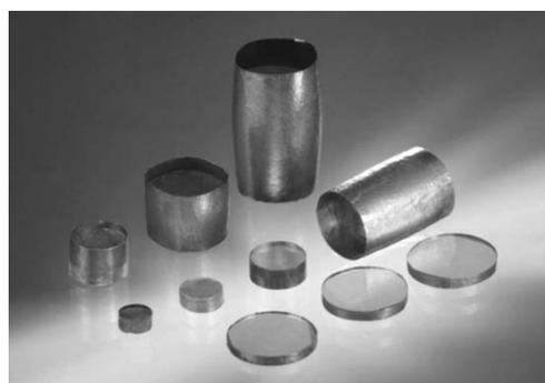
**Photo 1.** Nano-polycrystalline diamonds synthesized by direct conversion from graphite under high pressure and high temperature
