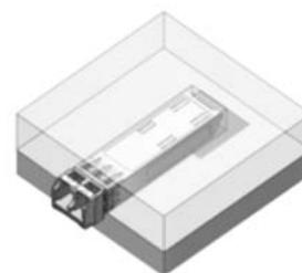
Fig. 6. Transceiver surrounded by metal
