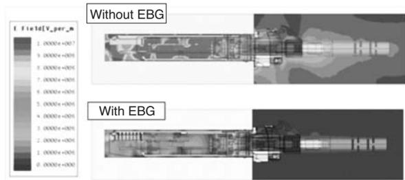
**Fig. 10.** Field distribution result of the transceiver with EBG. Above; without the EBG structure, below; with EBG structure. Red area indicates the field intensity is high. Although this result includes both near and far field, with corrugated structure shows the field distribution is “calm and quiet.”
