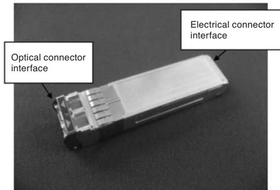
Fig. 1. External view of the optical transceiver "SFP+"
