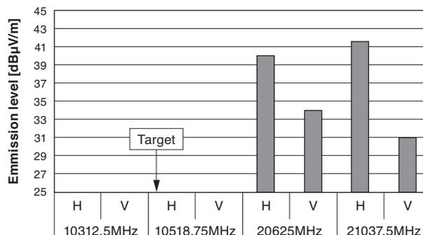
Fig. 7. EMI Result of the possible best shielding
