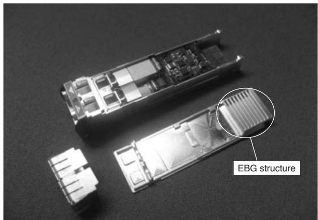
**Photo 1.** Photograph of the transceiver prototype with corrugated EBG chassis
