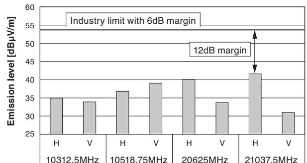
Fig. 2. EMI test result of the individual transceiver
