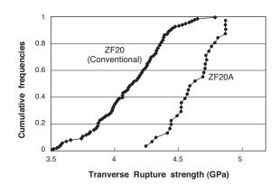
Fig. 12. Transverse rupture strength of ZF20A
