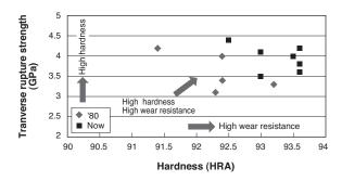
Fig. 10. Development of microdrill materials
