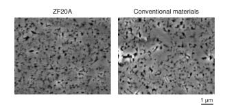
Photo 1. Microstructure of ZF20A
