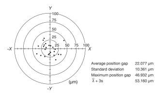
Fig. 6. Measurement of hole positioning accuracy
