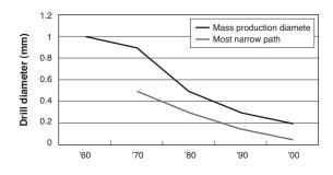
Fig. 3. Shifts in microdrill diameters
