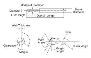
Fig. 2. Figures and names of microdrill parts
