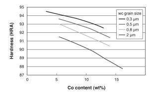
Fig. 8. Relations between Co content and hardness
