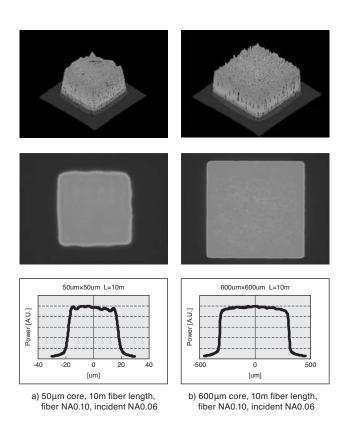
Fig. 6. Imaging patterns when multi-mode beams are incident
