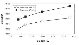
Fig. 4. Dependency of output NA on incident NA
