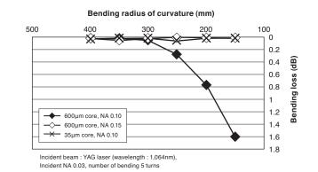
Fig. 3. Bending loss characteristics of rectangular core optical fibers
