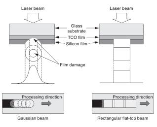
Fig. 2. Laser scribing in silicon thin film solar cells
