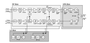
Fig. 3. Block diagram of analog block
