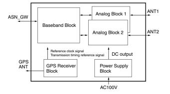
Fig. 1. Block diagram of prototype WiMAX base station
