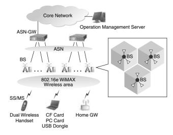
Fig. 6. WiMAX system configuration
