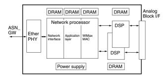
Fig. 2. Block diagram of baseband block
