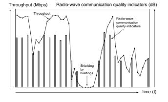
Fig. 8. Adaptive modulation measurement
