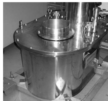
Fig. 15. Outer appearance of 8.1-T magnet
