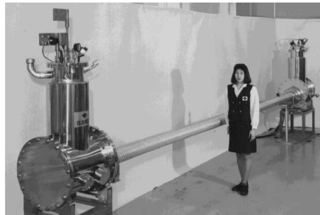
Fig. 20. 7-m-long "3-in-One" HTS cable prototype
