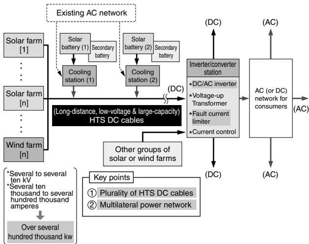
Fig. 22. GENESIS Project and HTS DC cables
