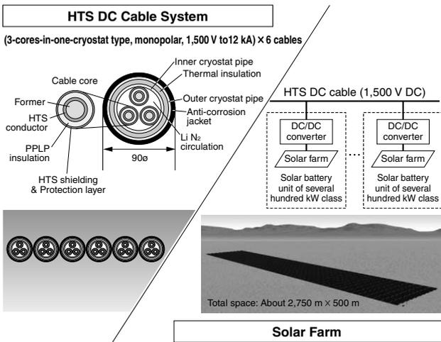
Fig. 28. 100-MW-class GENESIS System with HTS DC cable
