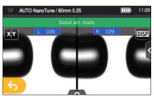
**3.** When the splicer shows "Good arc state", prepare fiber again to proceed to the splicing process. \*Fibers are not spliced in the arc test.
