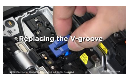
Replacing the V-groove
