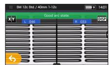
**3.** When the splicer shows "Good arc state", prepare fiber again to proceed to the splicing process. \*Fibers are not spliced in the arc test.
