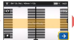
After "Arc Test Ready" appears, tap Set icon →. An arc test is started.
