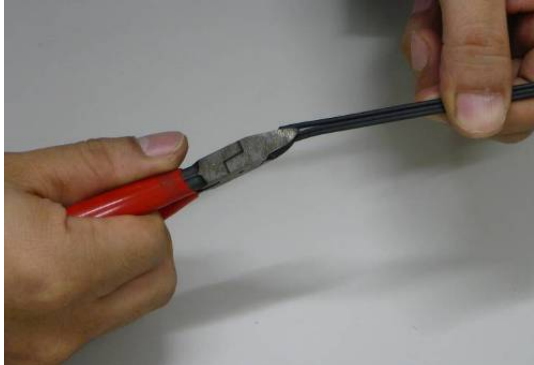
1: Separate the steel wire from the cable using nippers.
