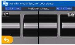
While splice program is selected to "AUTO NanoTune", the NanoTune™ analyzes the cleaved fiber surface and then sets up optimal splice condition.
