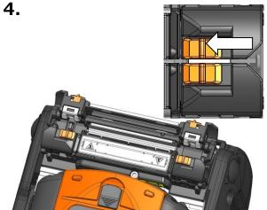
The heater clamp lid and heater lid move together by sliding the lever in the direction indicated by the arrow.
