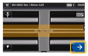
3: After "Arc Test Ready" appears, tap the Set icon → or press the Set key → An arc test is started.
