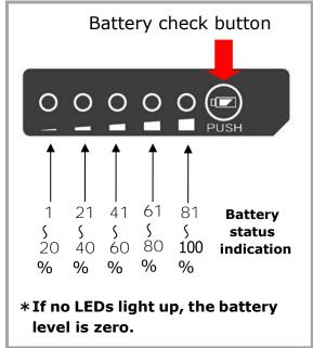
Check the battery level on the monitor
