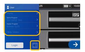
4: In Operator mode, splice program, heater program, function settings and sound setting cannot be edited.
