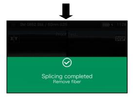
When the proof test is complete, the screen as shown above is displayed. Proceed with the heating process. See the next page.
