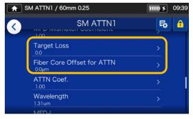
3: Select "Target Loss" or "Fiber Core Offset for ATTN" to edit the value.
