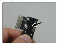
5: Load the cable in the fiber holder.Make sure that the cable sheath touches the groove.Close the bigger lid of the holder first, and then close the smaller lid.
