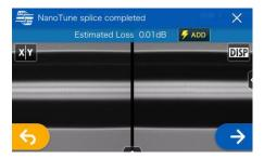
4: The NanoTune<sup>™</sup> splice is completed and an estimated loss is displayed.
