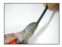
4: Make a slit along the groove of the cable sheath using nippers.
