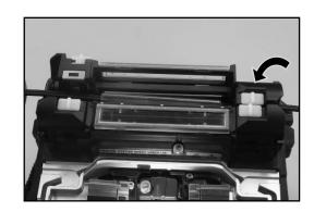
4: While applying a slight tension to the cable end, close the left hand oven clamp and oven lid. Start the heat shrink process.
