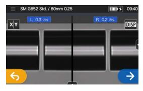
2: Inspection of fiber end face & dust.
