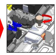
Splice performance is not stable or the splicer partly gets damaged if the electrodes are installed in a wrong way.
