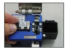
4: Place the fiber holder in the cleaver, touching the edge of the fiber holder against the edge of the fiber holder receptacle. Cleave the fiber referring to the cleaver instructions.
