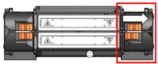
Slide the heater clamp lever in the direction indicated by the arrow.
