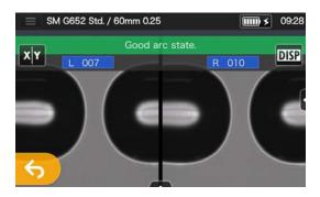
5: After "Good arc state." displayed, begin the fiber preparation procedure to perform a splice.
