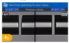
2: Inspection of fiber end face. The NanoTune™ is activated when the end face is poor.
