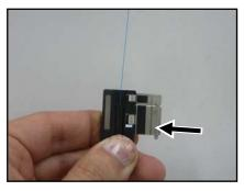
1: Load the cable with its sheath removed in the fiber holder. Make sure that the cable sheath touches the groove.
