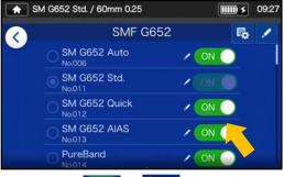
2: Tap ON OFF to switch between ON⇔OFF.
