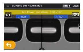
4: The melt back distance of the left and right fibers and the arc center position which are measured via image processing are displayed on the monitor screen. (The arc center position value is displayed only if the position is shifted.)
