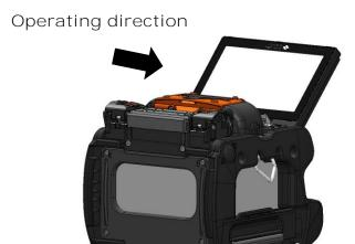
When the monitor is in the back position, your splicing work is easier if the right-hand and left-hand coating clamps are swapped. Refer to the following procedures.
