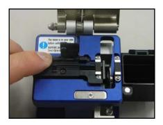
4: Place the cable in the groove for drop cable on the cleaver, aligning the cable end with the end of the single fiber adapter. Cleave the fiber referring to the cleaver instructions.
