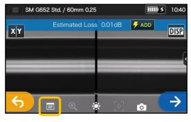
1: After splicing, tap the Splice data details icon ( ) on the Control panel ( ).
