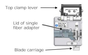
2: Lower the fiber straight into the correct groove of the single fiber adapter with the end of the fiber coating at the 16mm mark on the ruler (e.g. if the cleave length is 16mm).
