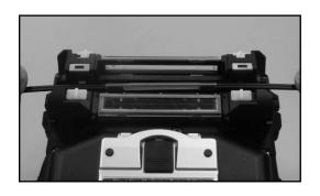
To keep excellent splice quality, regular cleaning and inspection are required. Especially cleaning should be performed before and after each use. We recommend your splicer to be checked through our maintenance service periodically.
