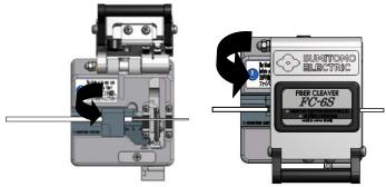
4: Slide the blade carriage to the rear of the cleaver as indicated by the arrow.
