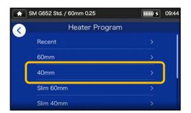
1: On the "Heater Program screen" (P.2-10), Select the sleeve type where you would like to change the settings.
