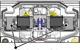
Coating clamp fixing screw
