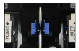
3: Make sure that the fiber sits in the V-groove correctly.
