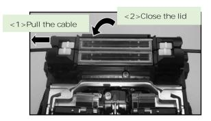
5: After the heat shrink process is complete, open the oven lid and oven clamps and take out the cable.
