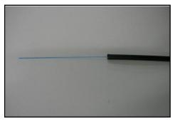
6: The cable sheath is removed. Repeat step 1 to 5 for the other cable. Cut each half of the cable sheath to the same length.
