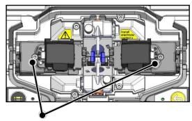
Coating clamp fixing screw
