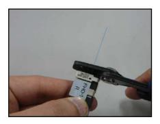
2: Remove the fiber coating at 2~4mm away from the edge of the fiber holder. (Touch the JR-M03 against the edge to remove, and you can remove the coating at 3mm away from the edge.)
