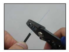
2: Remove the fiber coating from the mark using a jacket remover.
