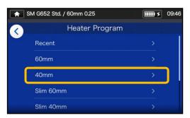
1: On the "Heater Program screen" (\*P.2-10), Select the sleeve type where you would like to change the settings.
