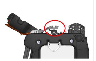
Slide the bare fiber pad release button in the direction indicated by the arrow.
