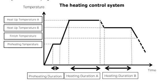
The heating control system is individually applied to each heater.
