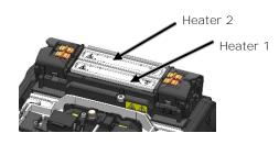
5: The Heater progress bar shows a progress of the heating cycle. The splicer gives a beep sound indicating completion of the heating cycle. Take out the sleeve from the heat shrink oven after a beep sound is heard.
