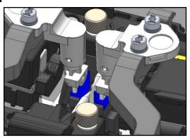
Make sure the bare fiber pad clamps the fiber properly.
