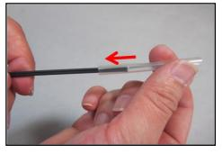
3: Insert a protection sleeve over the cable.
