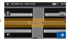
2. After "Arc Test Ready" appears, tap Set icon An arc test is started.
