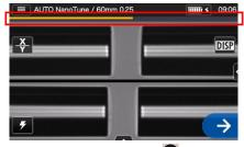
**5.** Press Heater key **(a)** to start the heating process. Heater progress bar
