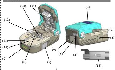
Fiber is cleaved and fiber offcut is collected along with opening and closing of the lid.
