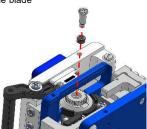
5: Remove the gear wheel and blade.
