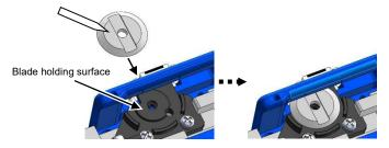
7: Re-insert the gear wheel back in the cleaver following the slotted part of the blade. Align the hole of the gear wheel with the hole of the blade.
