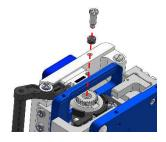
9: With "R Automatic rotation", slide the blade carriage to the rear of the cleaver. Ensure that the new blade is rotated 360 degrees in 24 steps.
