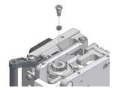
9: With "R Automatic rotation", slide the blade carriage to the rear of the cleaver. Ensure that the new blade is rotated 360 degrees in 24 steps.
