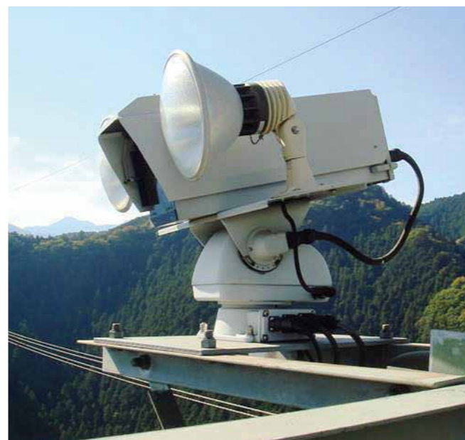
Controllable camera for monitoring overhead lines
