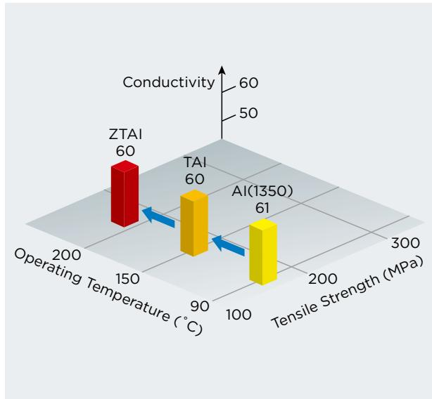
Thermal-resistant aluminum alloy (TAI) and Super thermal-resistant aluminum alloy (ZTAI) improve its thermal-resistant characteristics by adding zirconium. ZTAI and TAI can keep its tensile strength in high temperature condition.
