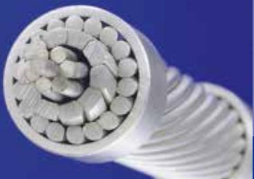
GTACSR/GZTACSR has a unique construction featuring a small gap between the steel core and (Super) Thermal-resistant aluminum alloy layer. The combination of the (Super) Thermal resistant aluminum alloy and the "Gap construction" offers excellent sag and current-carrying characteristics. With this advantage, GTACSR/GZTACSR is useful to up-rate an existing transmission line by simply replacing the existing conductor to GTACSR/GZTACSR.
