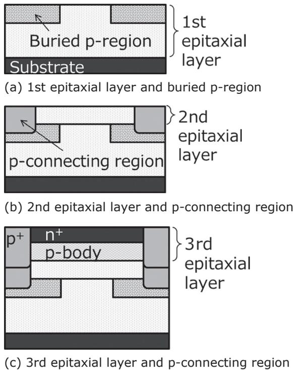
Fig. 2. Fabrication process for SiC VMOSFET
