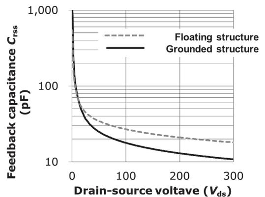
Fig. 4. Capacitance characteristics of SiC VMOSFET
