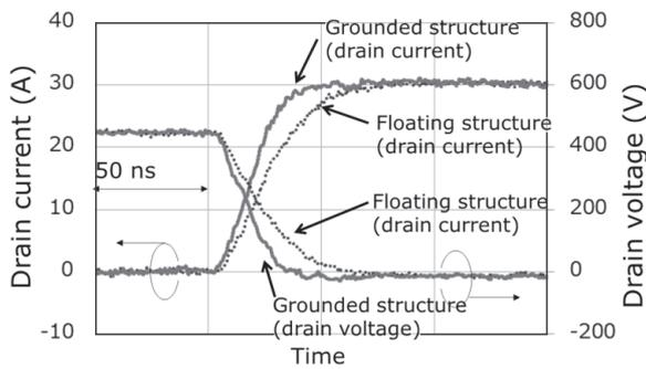
Fig. 6. Turn-on switching waveforms
