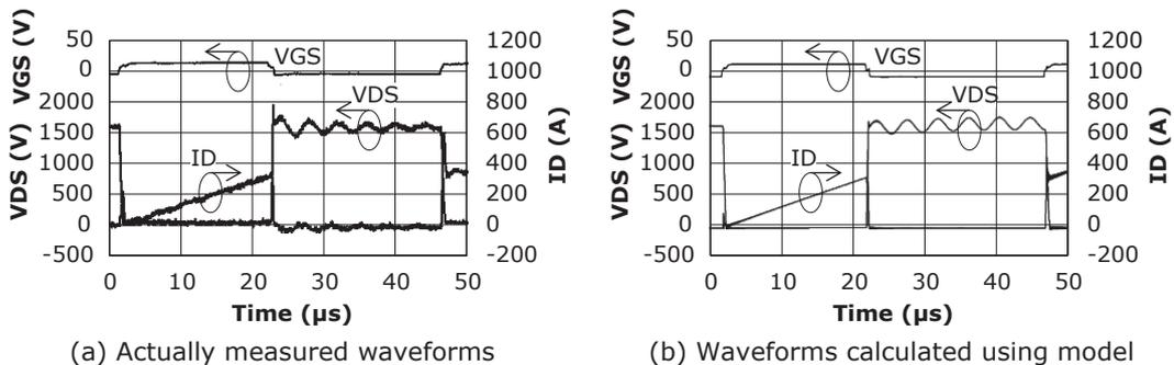
Fig. 8. Comparison of dynamic characteristics waveforms (switching of inductance load at power source voltage of 1,650 V)
