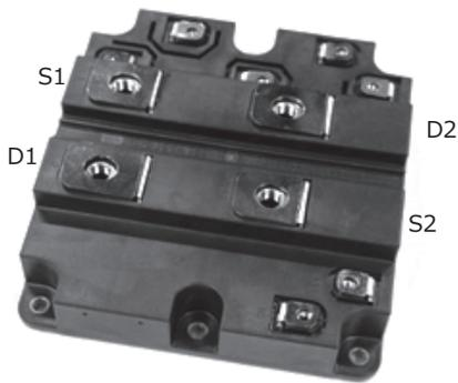
Fig. 1. 3,300 V, 400 A 2 in 1 SiC power module (130 x 140 mm<sup>2</sup>)
