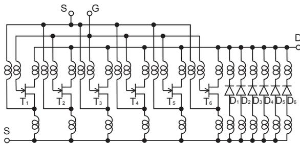
Fig. 6. Equivalent circuit of module (for a single substrate)
