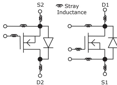
Fig. 4. Equivalent circuit of a previous module
