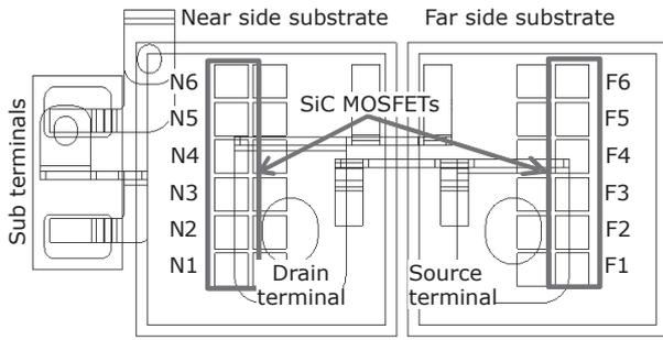
Fig. 9. Chip layout for one arm
