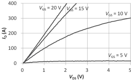
Fig. 2.  $I_D$ - $V_{DS}$  forward characteristics of 3,300 V, 400 A SiC power module
