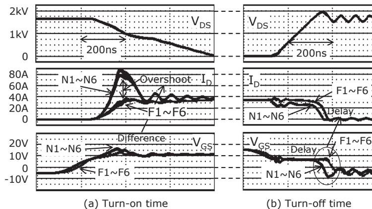
Fig. 10. Calculated switching waveform of each chip current (power source voltage: 1,650 V)
