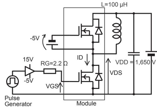
Fig. 7. Dynamic characteristics evaluation circuit
