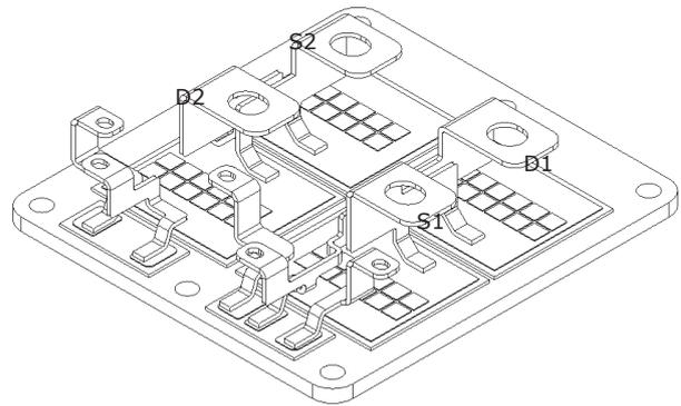
Fig. 3. Internal structure of 3,300 V, 400 A SiC power module
