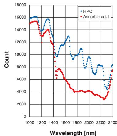
**(c) Reflectance spectra of hydroxypropyl cellulose (HPC) and ascorbic acid**
