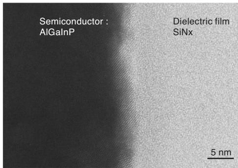
**Photo 1.** Transmission electron microscope (TEM) image of interface between dry etched AlGaInP surface and SiNx film
