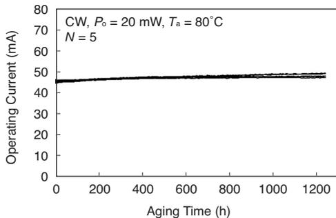
Fig. 6. Reliability test result under 20-mW CW operation at 80°C
