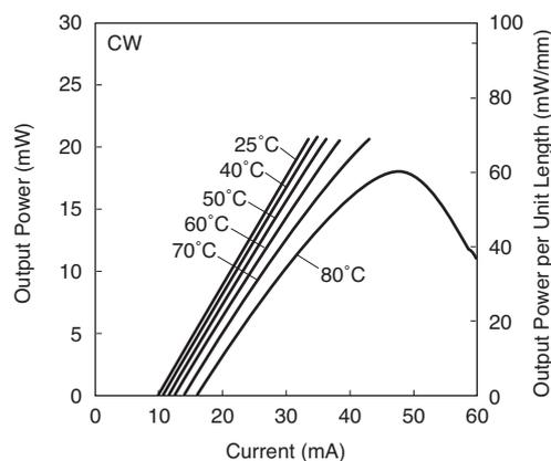
Fig. 4. Temperature dependence of  $L-I$  characteristics ( $L = 300 \mu\text{m}$  LD, CW operation)
