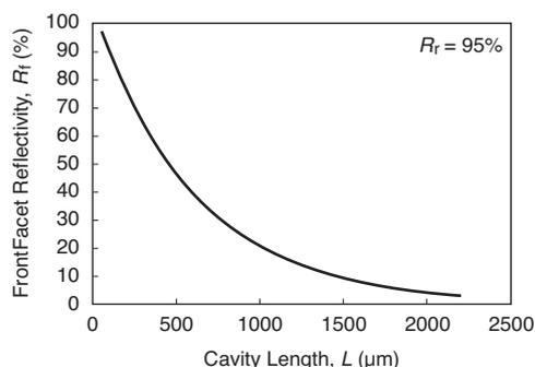
Fig. 3. Dependence of front facet reflectivity  $R_f$  on cavity length  $L$  with constant  $J_{th}$
