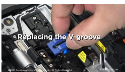
Replacing the V-groove
