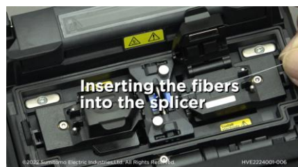
Inserting the fibers into the splicer
